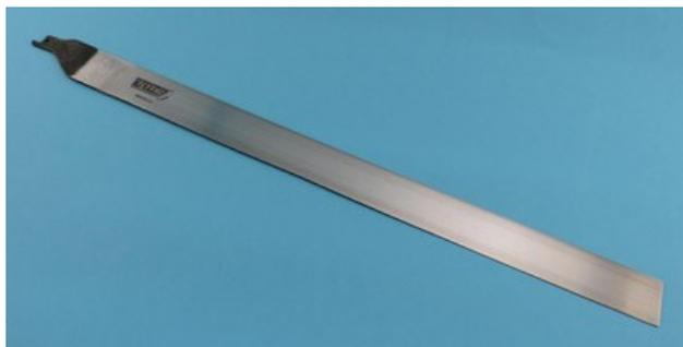
Fitting into a standard reciprocating saw with a 1/2" tang, the new Spray Foam Insulation Reciprocating Saw Blade measures 19" in overall length with a long 16" cutting length. This double bevel, straight-edged blade is constructed of high carbon steel and is coated with a glazed finish to prevent sticking when cutting foam that has expanded into unwanted areas. The Spray Foam blade and its tang are hardened for long life and improved operator safety in use.
