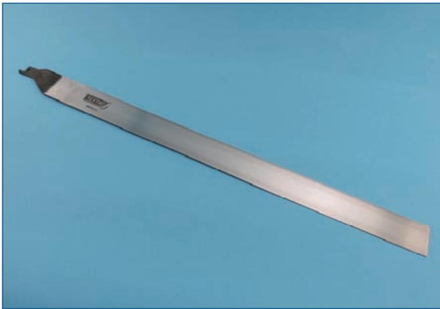
We start with a high carbon steel blank, then grind it, heat treat it and temper it to the high standards you demand. With a 1/2" universal tang, the spray foam insulation blade fits all common reciprocating saw machines. The induction hardening of the tang end of the blade provides the flex you need in the shop or cutting up against framing studs.
